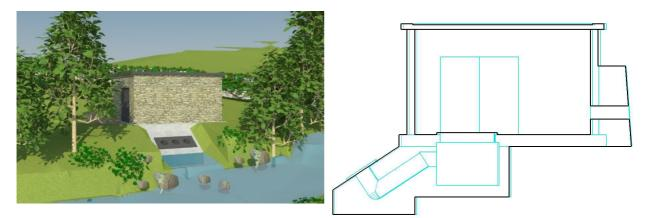
Figure 7: Acoustic isolation of the hydropower equipment is possible through the introduction of an airlock in the tailrace pipes as illustrated
