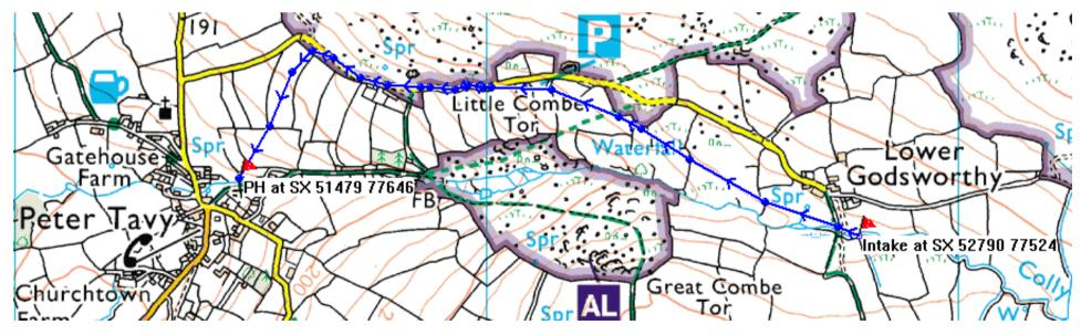
Figure 1: Ordnance Survey map showing proposed location of intake, powerhouse and pipe route
